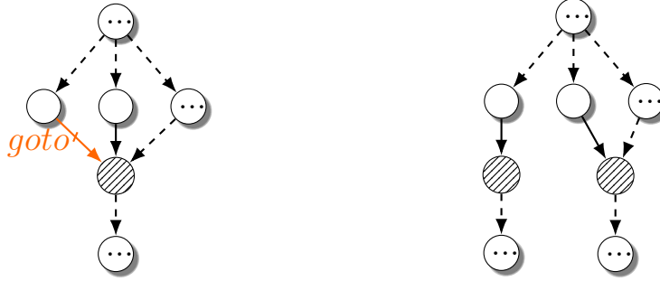
Figure 2.6: CFGs before and after deoptimizing an ISC optimization case. ISC cases contain a goto edge connecting one node to another node that has multiple predecessors. Duplication of the shaded node, and all its single-successor ancestors, revert this case.
